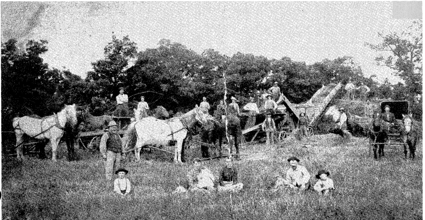
THIS PHOTO of an early grain separator (threshing) machine was taken near Center Junction in August 1888. Six teams are hooked to a 12-horsepower machine. The man feeding
